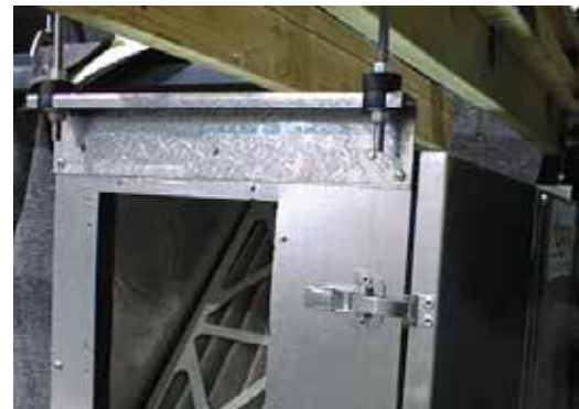
Figure 3. Unit hung from ceiling using optional hanging bracket kit, 45EVHB. To install hanging bracket, identify the corners of unit you wish to hang it from. Remove existing screws from unit pan. Attach hanging bracket to unit using screws provided with the hanging bracket
