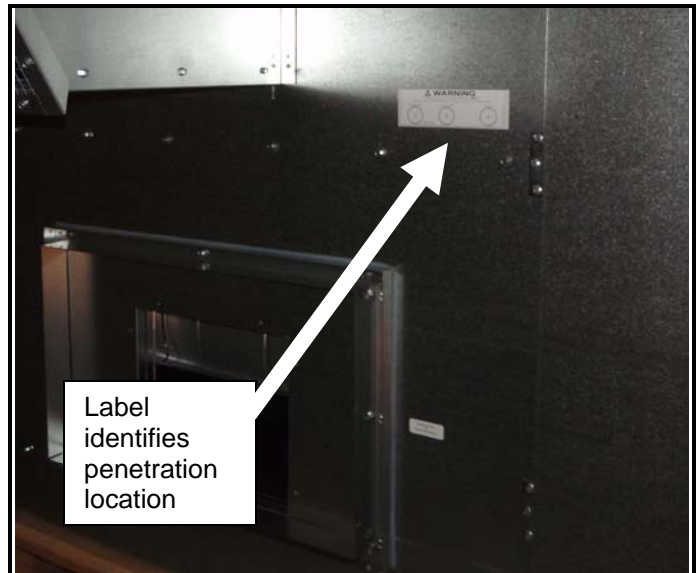
FIGURE 4-6 WIRE ENTRY THROUGH OUTLET SIDE OF UNIT
