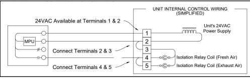
FIGURE 5.5.2 EXTERNAL CONTROL USING ERV 24 VAC
