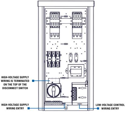
FIGURE 5.3.0 E-BOX\_WIRING ENTRY POINTS
