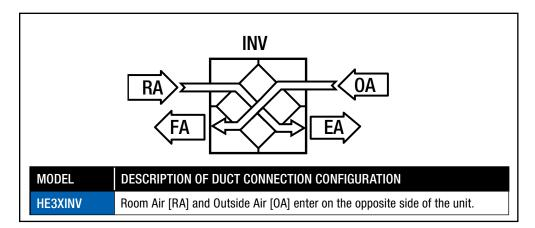
**FIGURE 1.2.0 AIRFLOW ORIENTATION**
