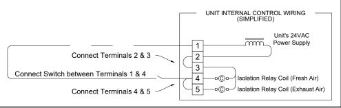
FIGURE 5.5.0 SINGLE 2-WIRE CONTROL, UNPOWERED
