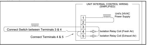
FIGURE 5.5.1 24 VAC FROM EXTERNAL SOURCE
