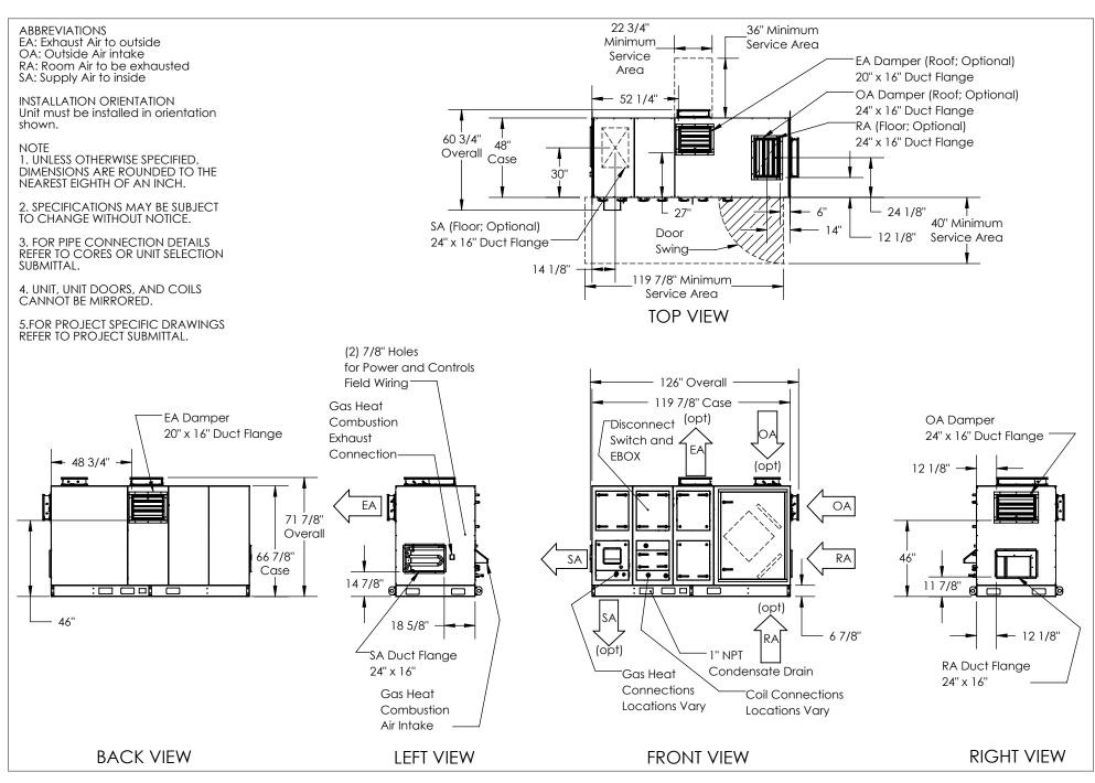
Model: DN-2JIN ERV+COIL+HEAT 1" Drawing Type: Unit Dimension Version: NOV18
