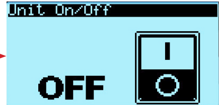
Click UP or DOWN Arrow Button to Change Status to ON. Click the ESCAPE Button to Return to the Main Menu.
