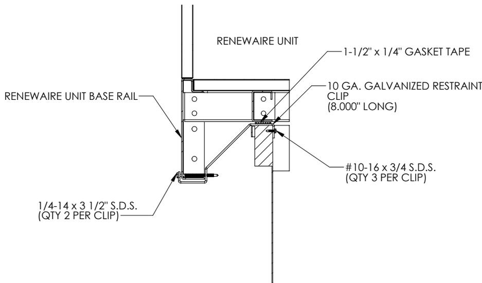
FIGURE 2.6.1 DN3 ERV ONLY CURB CLIP INSTALLATION
