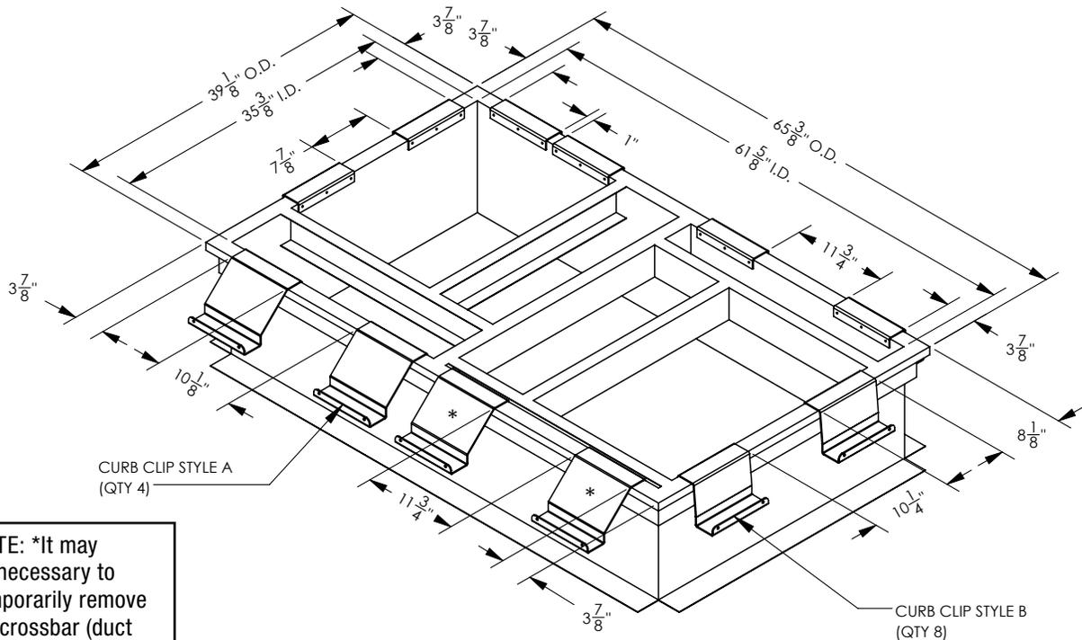
FIGURE 2.3.0 DN2 ERV ONLY CURB CLIP PLACEMENT
