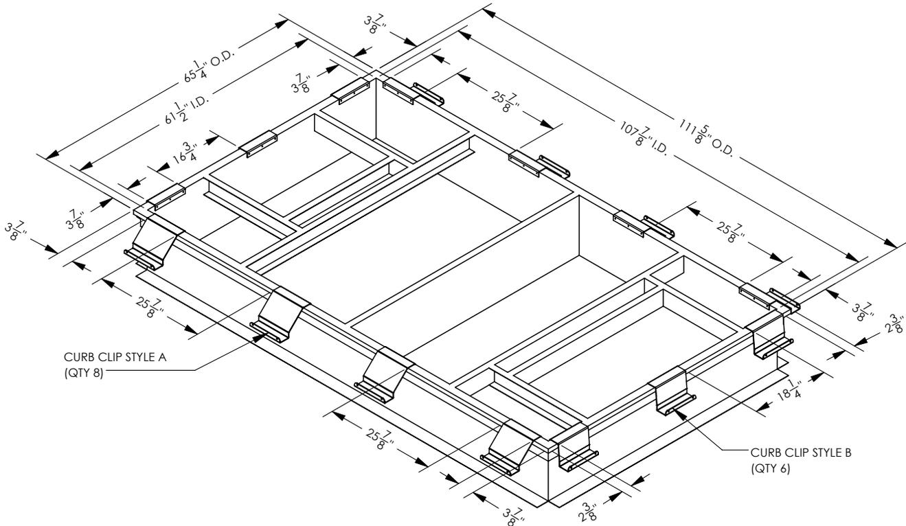
FIGURE 2.8.0 DN3 ERV+HEAT CURB CLIP PLACEMENT
