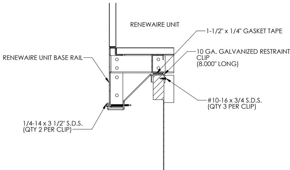
FIGURE 2.10.1 DN5 ERV ONLY CURB CLIP INSTALLATION
