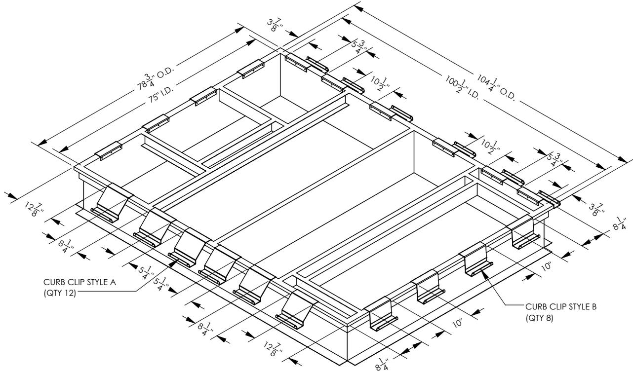
FIGURE 2.11.0 DN5 ERV+COIL CURB CLIP PLACEMENT
