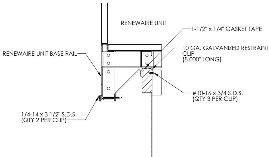
FIGURE 2.4.1 DN2 ERV+COIL OR HEAT CURB CLIP INSTALLATION
