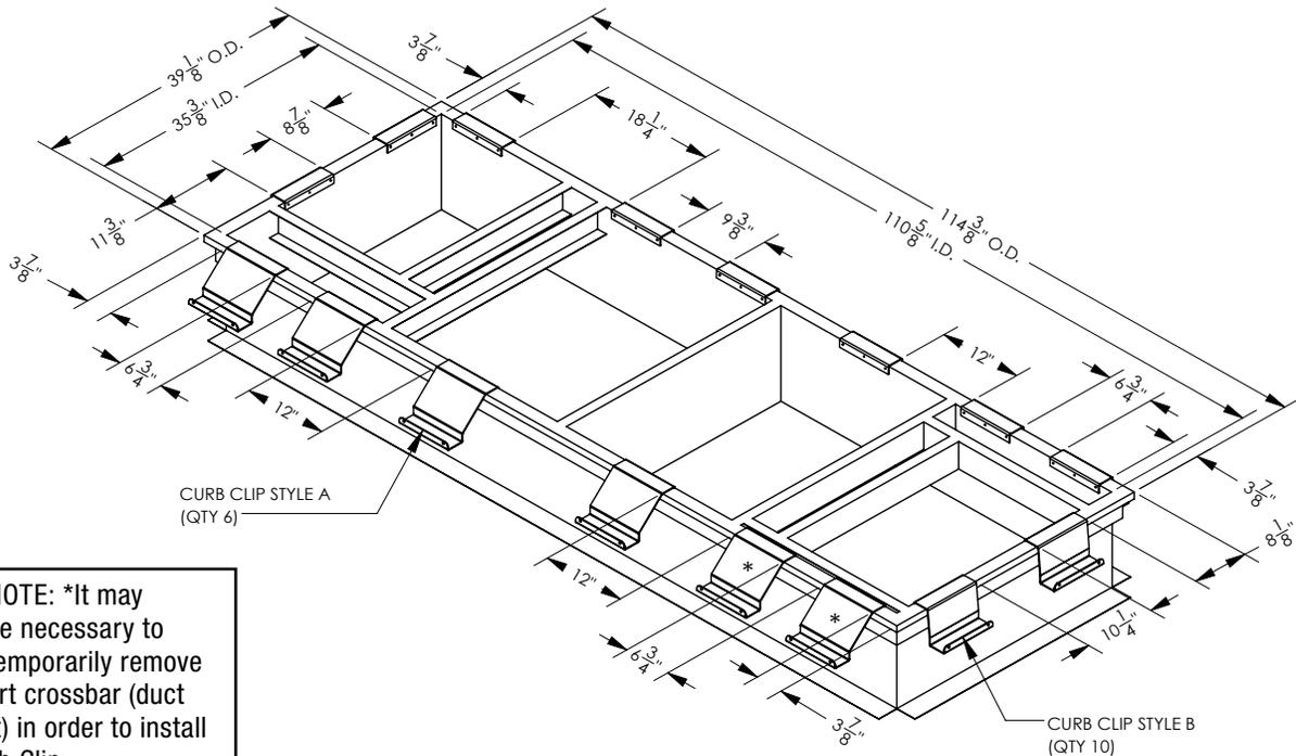
**NOTE:** \*It may be necessary to temporarily remove the short crossbar (duct support) in order to install the Curb Clip.
