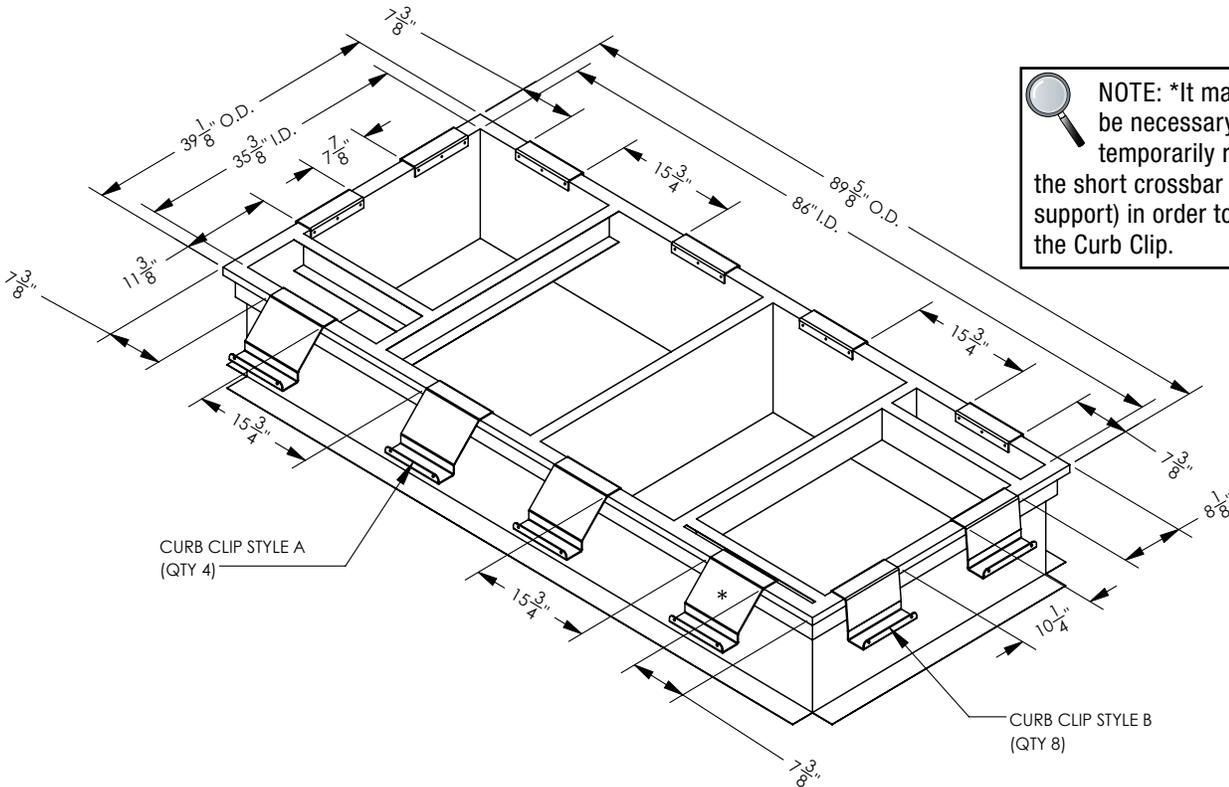
FIGURE 2.4.0 DN2 ERV+COIL OR HEAT CURB CLIP PLACEMENT
