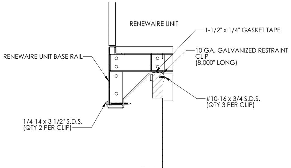
FIGURE 2.5.1 DN2 ERV+COIL+HEAT CURB CLIP INSTALLATION
