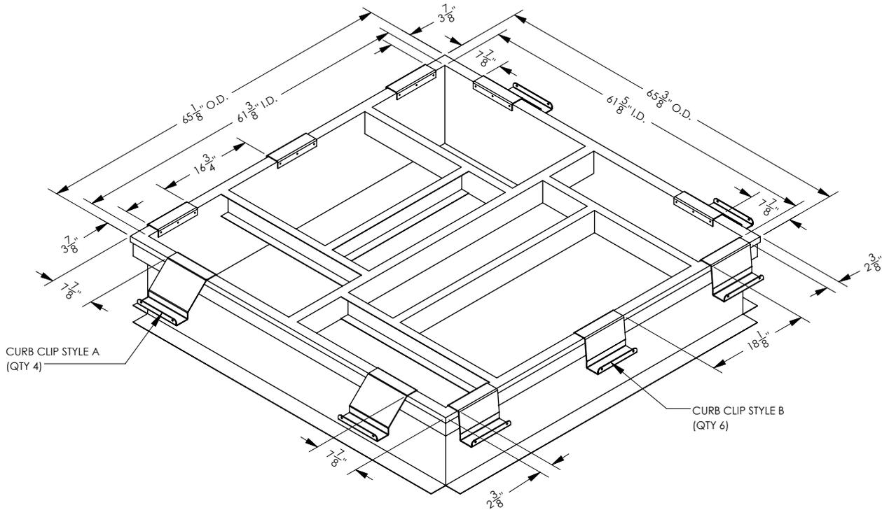
FIGURE 2.6.0 DN3 ERV ONLY CURB CLIP PLACEMENT
