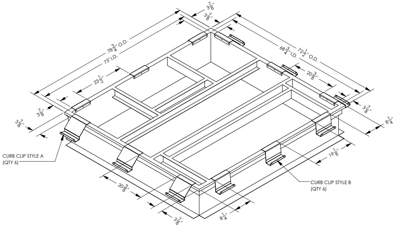
FIGURE 2.10.0 DN5 ERV ONLY CURB CLIP PLACEMENT
