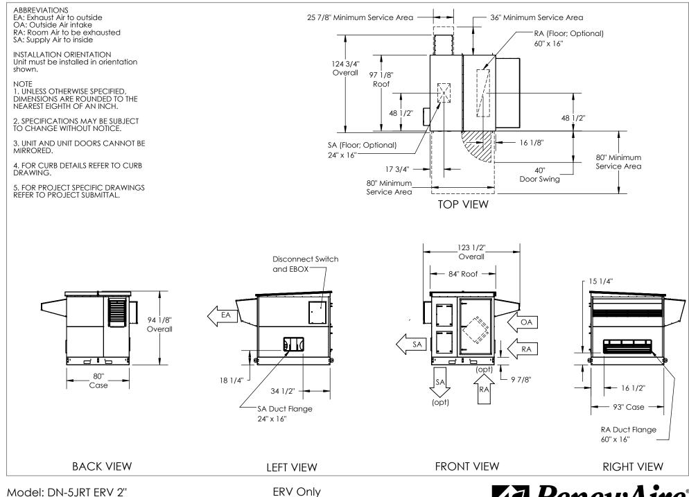
Model: DN-5JRT ERV 2" Drawing Type: Unit Dimension Version: DEC18 ERV Only No Coils, No Heat
