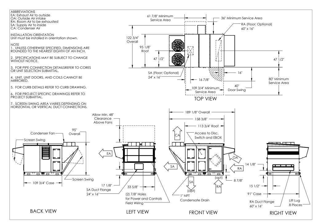
Model: DN-5JRT-PKGD ERV+COIL 1" Drawing Type: Unit Dimension Version: JUN20
