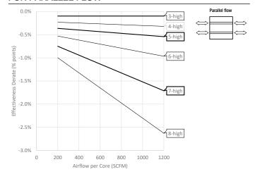
When parallel flow airflow orientation is used, flow is not optimally distributed to every exchanger and performance is slightly reduced. In this case the sensible and latent effectiveness must be derated by the amount shown in the EFFECTIVENESS DERATE chart. This derate is automatically applied by CORES.RenewAire.com (v1.3.0 and after) when parallel flow orientation is selected.
