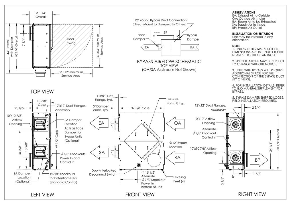
Model: HE07INH [Bypass] Drawing Type: Unit Dimension Version: AUG23
