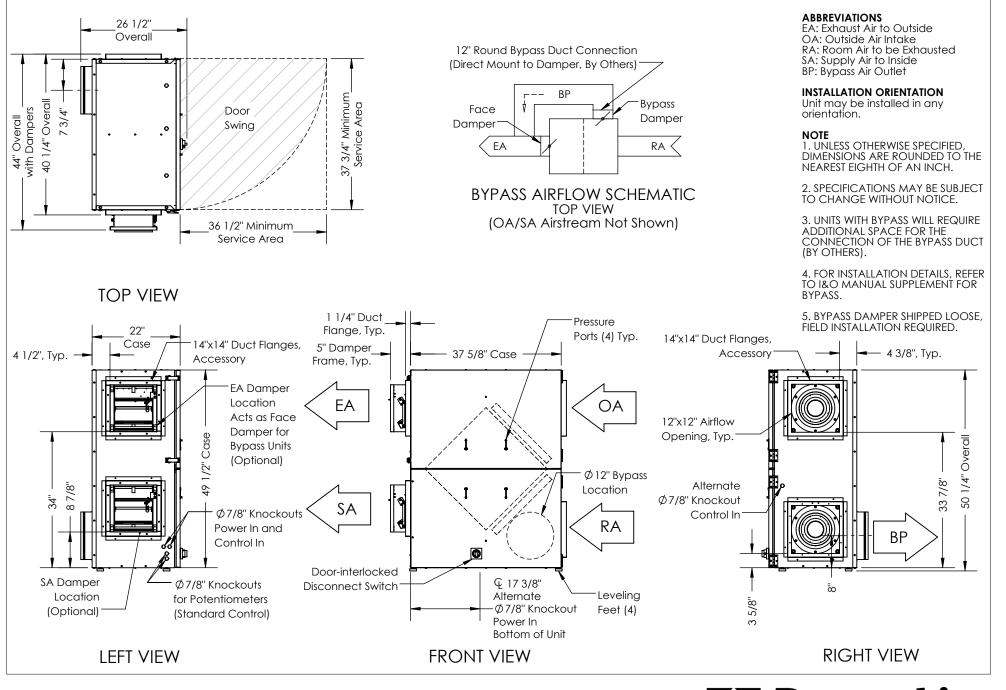
Model: HE10INH [Bypass] Drawing Type: Unit Dimension Version: AUG23 RenewAire® Energy Recovery Ventilation
