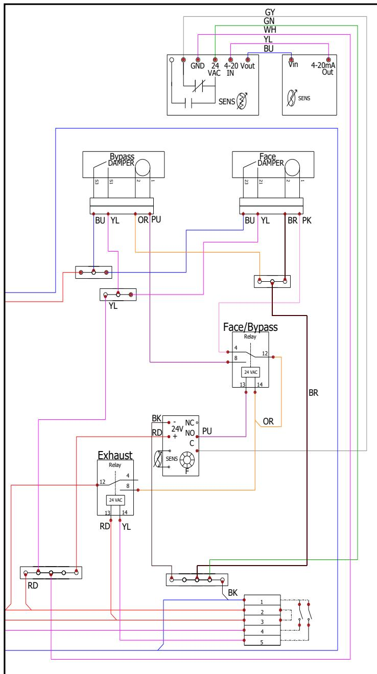
FIGURE 5.2.0 ENTHALPY CONTROL WIRING SCHEMATIC
