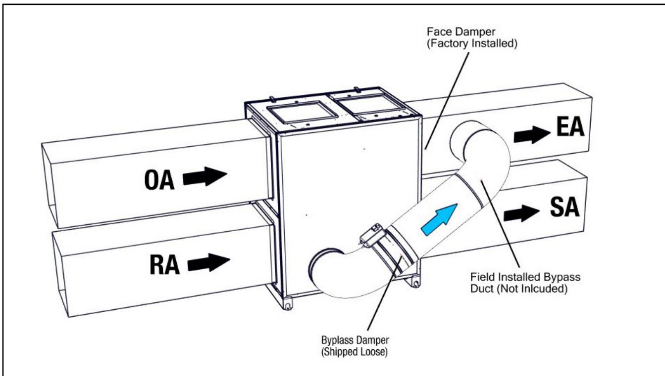
FIGURE 1.1.5 TYPICAL ERV WITH CORE BYPASS
