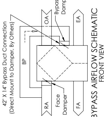
**BYPASS AIRFLOW SCHEMATIC
