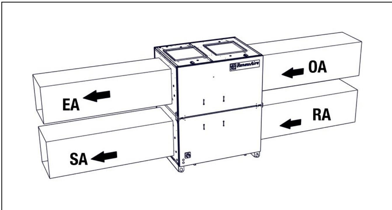
FIGURE 1.1.4 TYPICAL ERV WITHOUT CORE BYPASS
