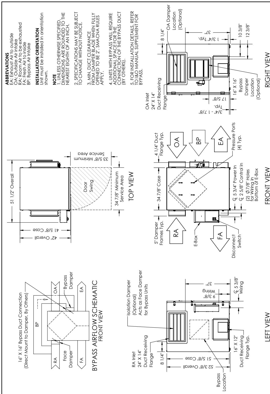
FIGURE 5.6.1 HE2XINV DIMENSION DRAWING (VERTICAL AIRFLOW ORIENTATION)
