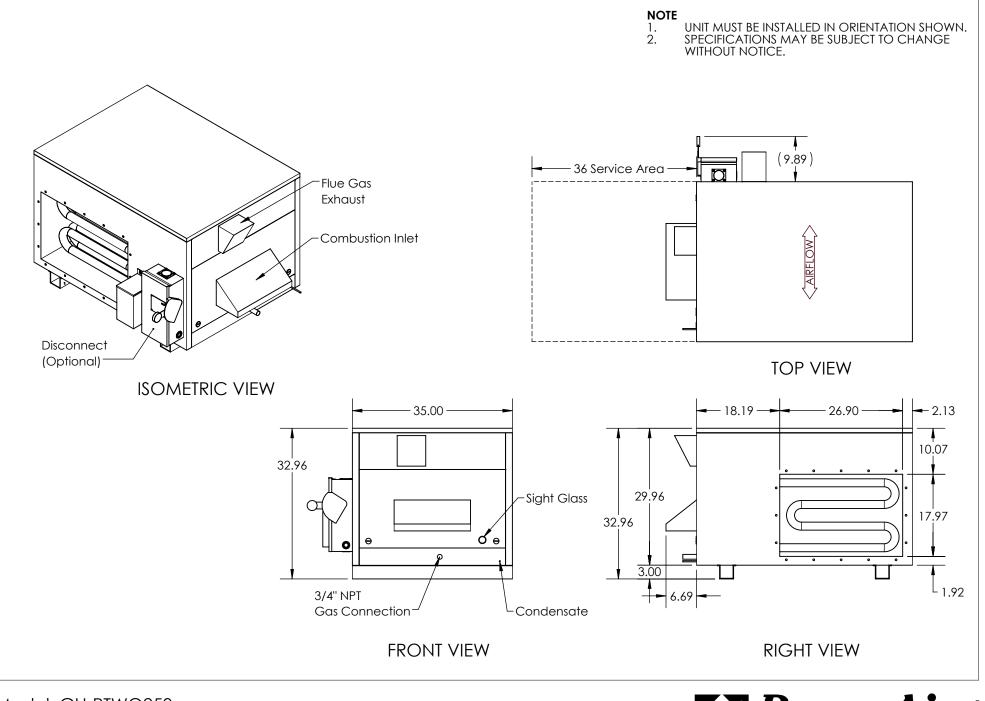
Model: GH-RTWO250 Drawing Type: Unit Dimension Version: OCT23 **RenewAire**<sup>®</sup> Energy Recovery Ventilation
